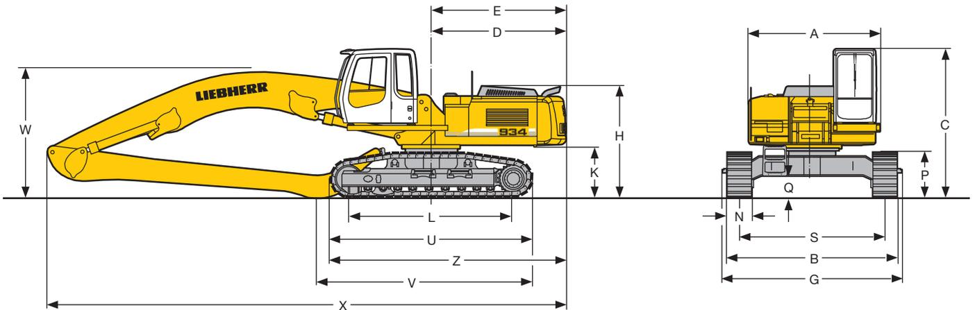
These dimensions are stated with cab carrier. This assembly is only valid for transportation.
